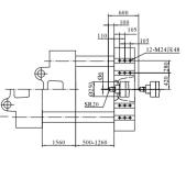
For UN850W1 and UN1100W1, the outmost ejector pins marked in the drawings are standard either in the horizontal or vertical direction. (Two directions can not be standard at the same time)
