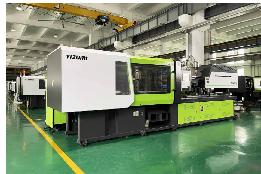
Electric injection molding machine workshop at YIZUMI
