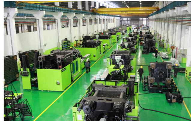
■ Two-platen injection molding machine assembly workshop at YIZUMI
