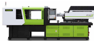
FF120 series electric injection molding machine
