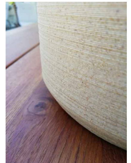
Picture 3: Side wall of a printed part made of Biofibre Silva Si2900
