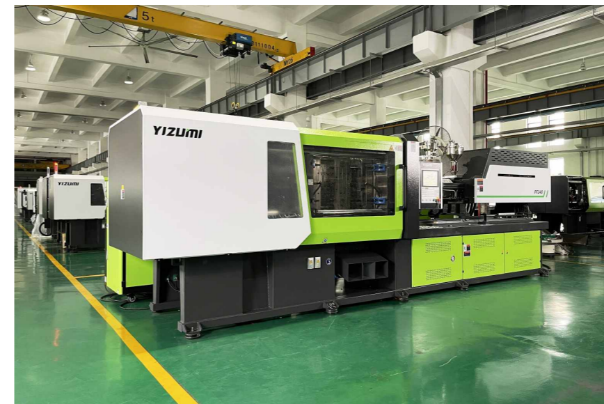
Electric injection molding machine workshop at YIZUMI
